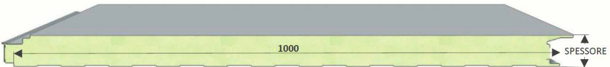
FIGURE 1 –ISOPARETE PANEL FACER PROFILES
